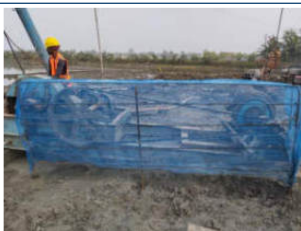
Safety Guard for Rotating Equipment
