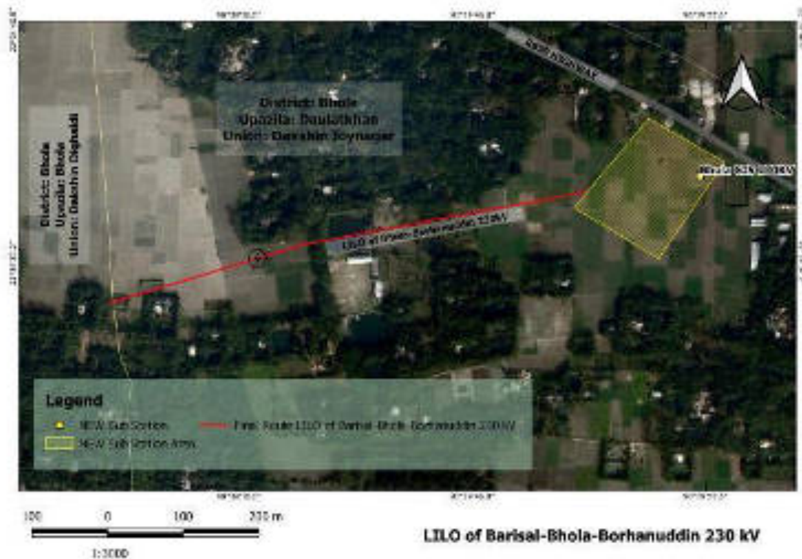
Figure 28: LILO Connection to Bhola Substation
