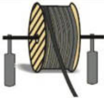
Figure 3-3: Placement of cable drum and correct method of pulling
